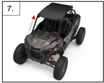
Re-torque all the fasteners after 100 miles.
